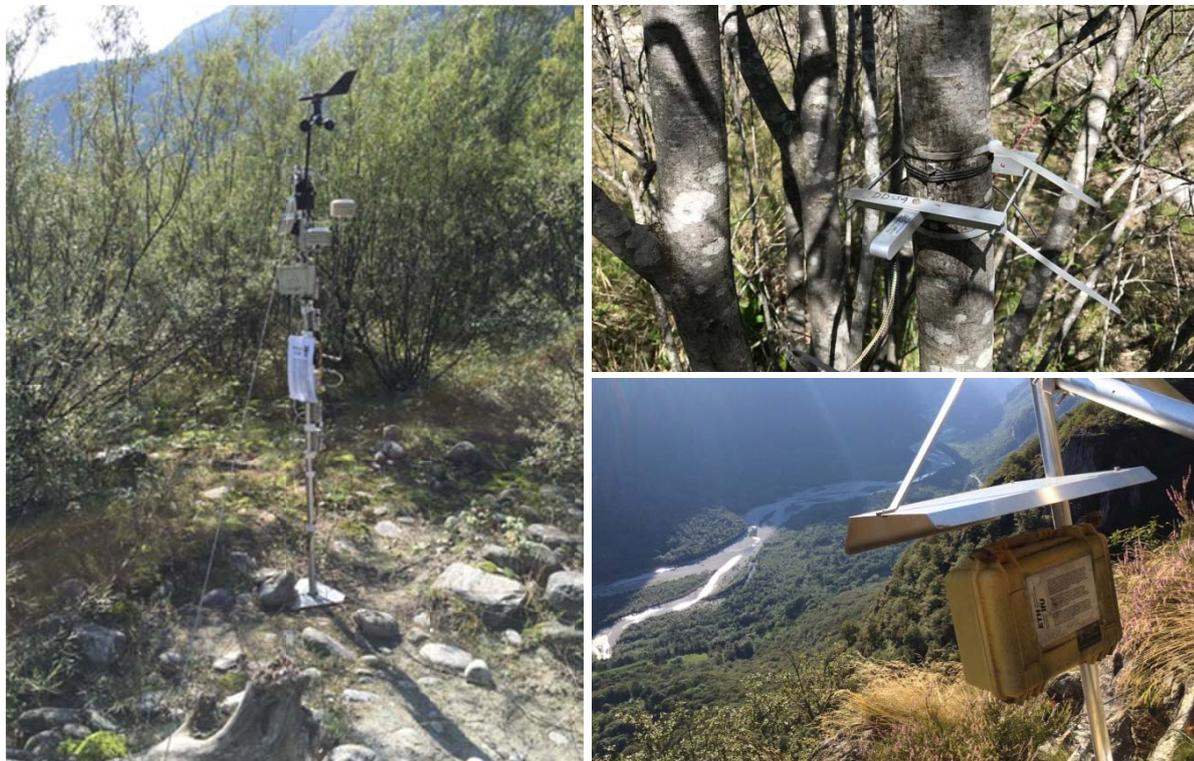
**Figure 6:** Weather station, dendrometer and camera used for measurements in the main valley (©Gianluca Bergami)
