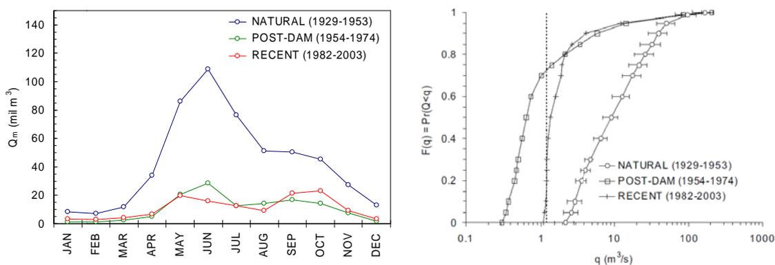
**Figure 5:** Mean monthly streamflow in Bignasco before and after dam construction (left) and the cumulative probability distribution of daily streamflow in the pre- and post-dam periods (right).
