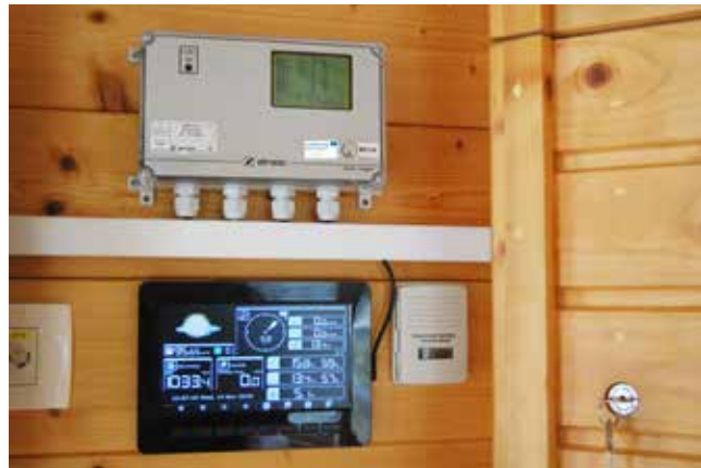
A display in log cabin (above) shows the temperatures of shallow subsoil at a depth of 10 cm, 50 cm, and one meter below surface.
