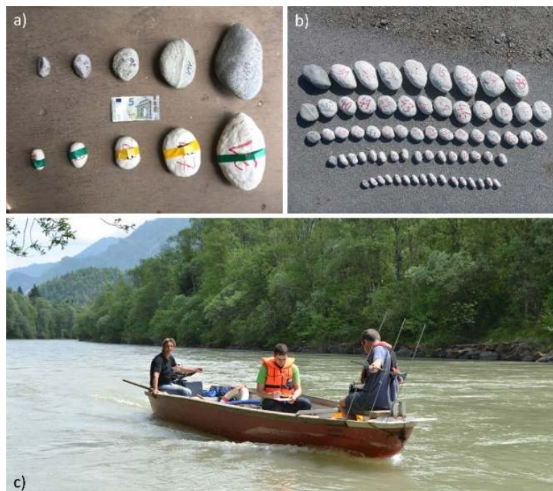
Figure 1. a) and b) Bedload tracers (active VHF transmitters) deployed in the Upper Drava valley, c) search of tracers with a mobile radio receiver and antenna from a boat.
