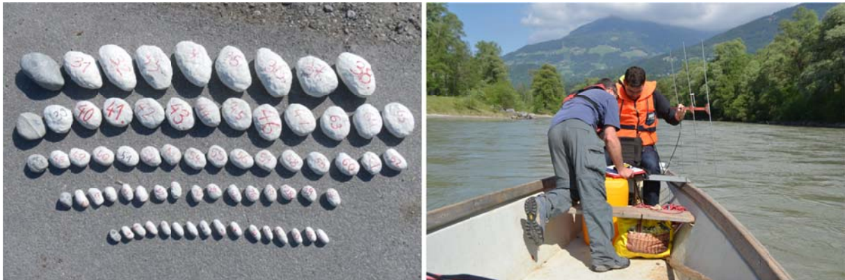
Figure 11: 65 coded radio tracer stones implemented in the Drau River (left) and the process of searching the tracers by boat
