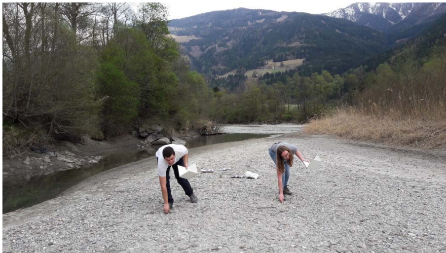
Figure 10: Sediment sampling for grain size analysis based on Wolman pebble counts
