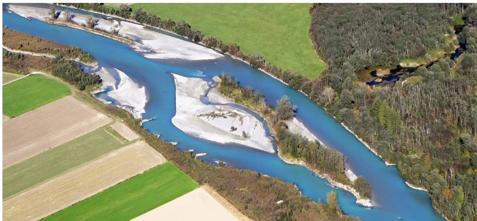
Figure 7. Upstream part of the restored reach near Obergottesfeld in 2017. Massive riverbank erosion required the installation of additional bank protection (groynes) to prevent the erosion of private property. Flow is from right to left (image source: Carinthian government).
