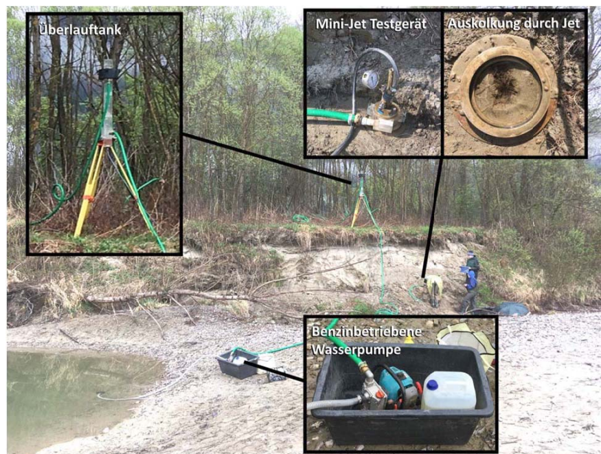
Figure 12: Experimental setup of the jet test
