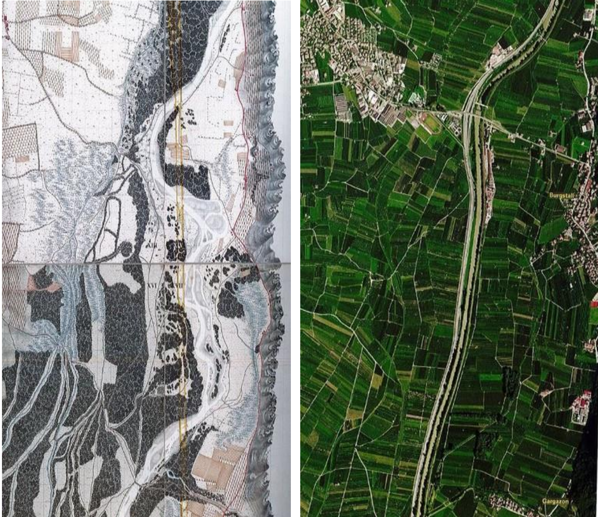
Figure 3 - Adige at Postal (Burgstall in German) at the beginning of 1800 (left) and in the 1998-1999 (right). The yellow lines on the left image indicate the river channelization proposal of the Austrian military engineer Ignaz von Nowack
