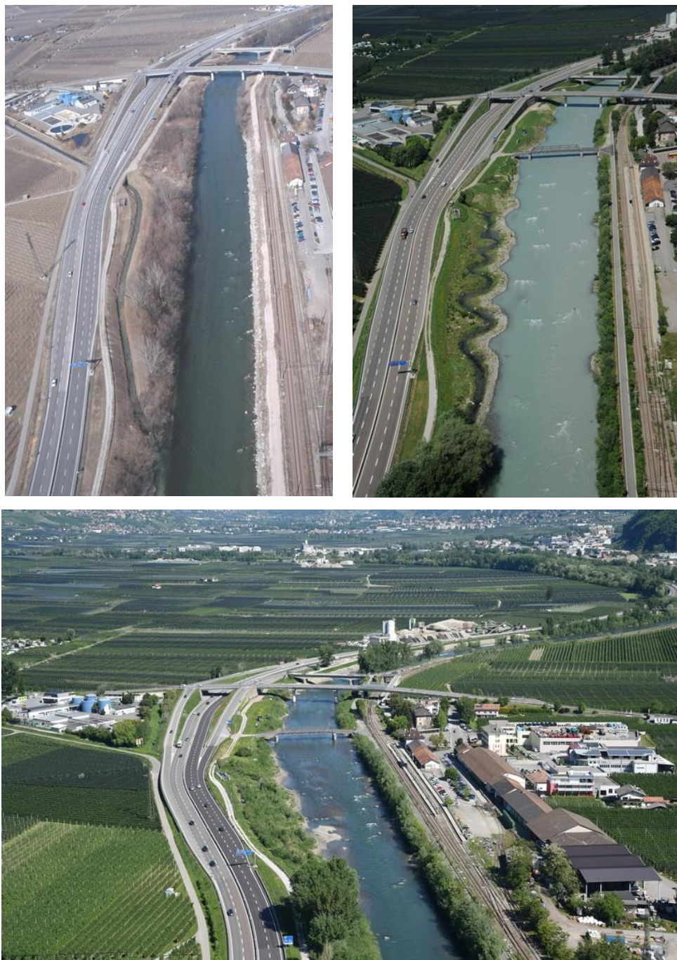
Figure 6 - Adige River at Postal. River reach before the restoration on the top-left (2009), and after the restoration in 2013 on the top-right and in 2016 on the bottom
