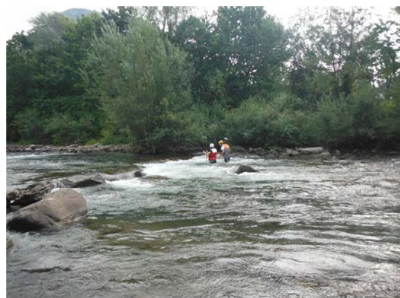
(f) Measurements taken during a discharge of 6.4 \text{ m}^3/\text{s}
