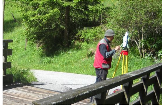
(b) TS used for collecting topographic data
