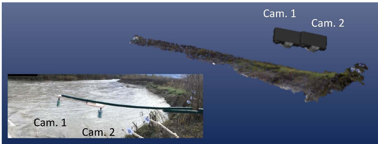
Figure 30. Test of using two time-lapse cameras for continuous monitoring of riverbank geometry.
