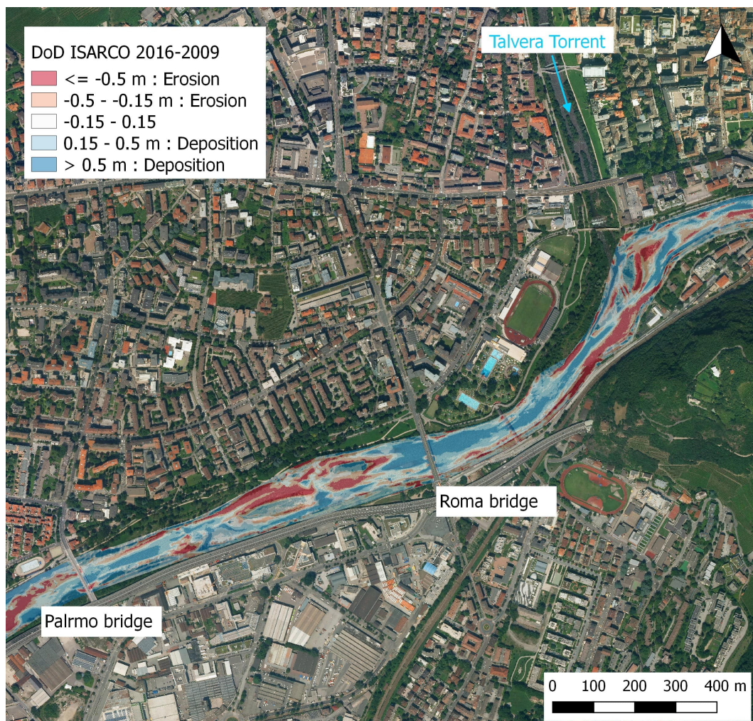
Figure 19: Overview of the DoD 2016–2009 computed for the study reach at Roma bridge; water flows from right to left
