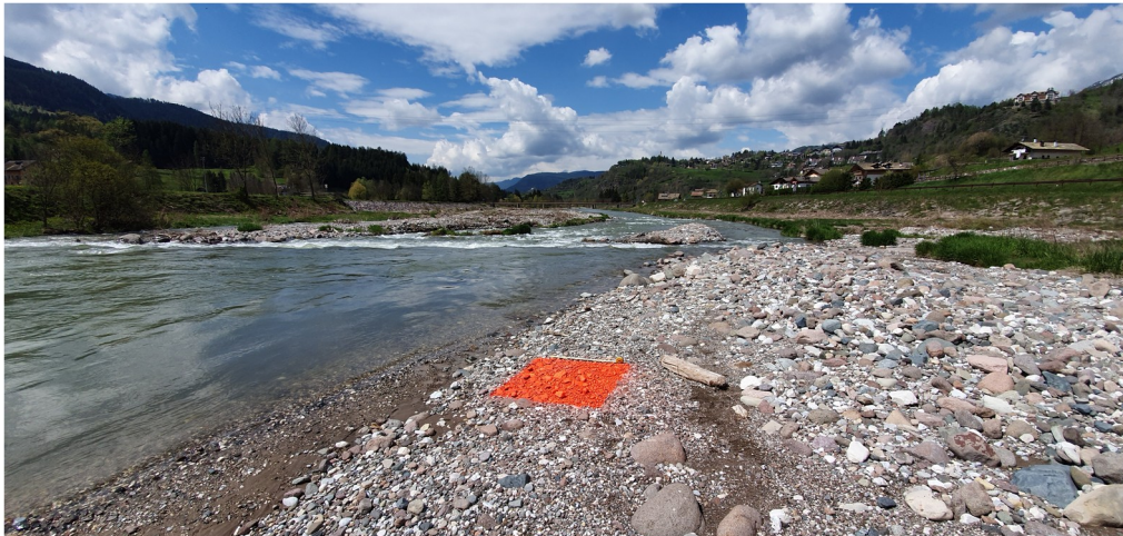
Fig.5. Painted gravel plot to investigate bedload initiation.
