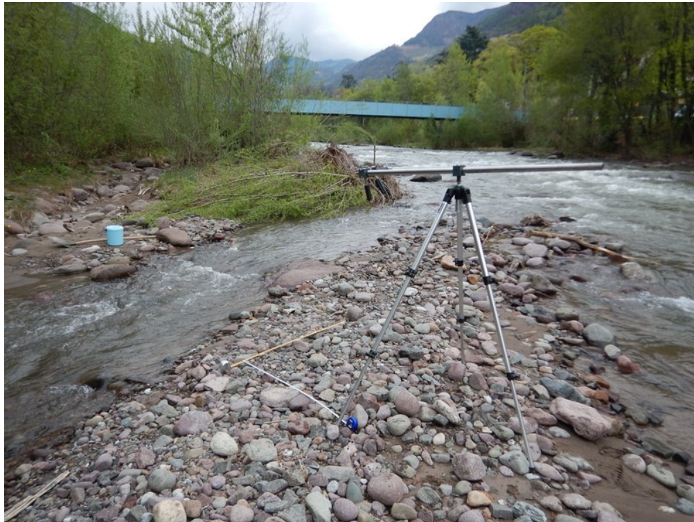
(a) Identification of the sampling area and positioning of the mount supporting the camera
