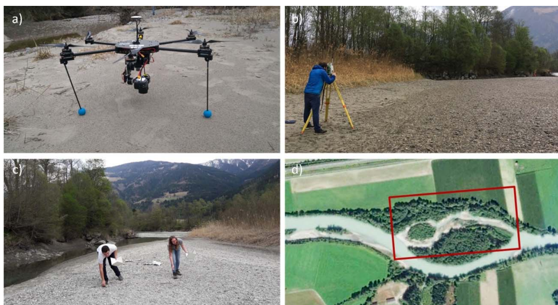
Figure 6. Morphological monitoring at the Drau River (Austria) - a) used drone for the structure from motion (SfM) photogrammetry, b) terrestrial survey, c) Wolman pebble counts for grain size analysis, d) location of the survey
