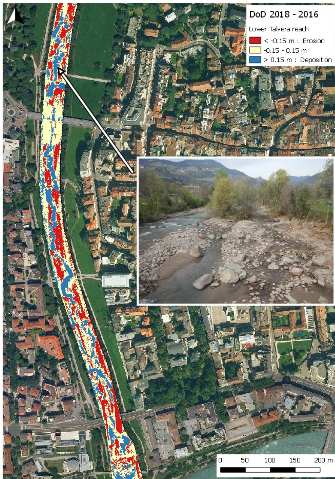
Figure 31: DoD 2018-2016 of the low study reach of the Talvera Torrent with a picture showing a deposition area
