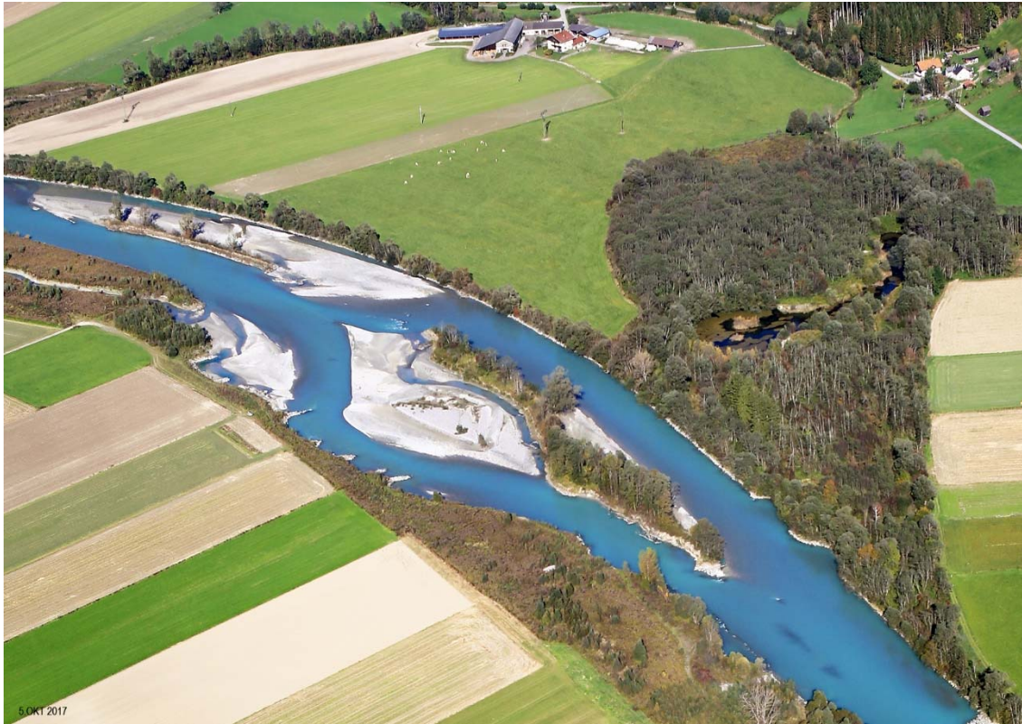
Figure 2. Emergence and enlargement of a mid-channel bar at a restored site of the Drau River, accompanied by excessive widening which required an expansion of bank protection (groynes) to prevent erosion of land outside of the provided corridor (source: Carinthian government).
