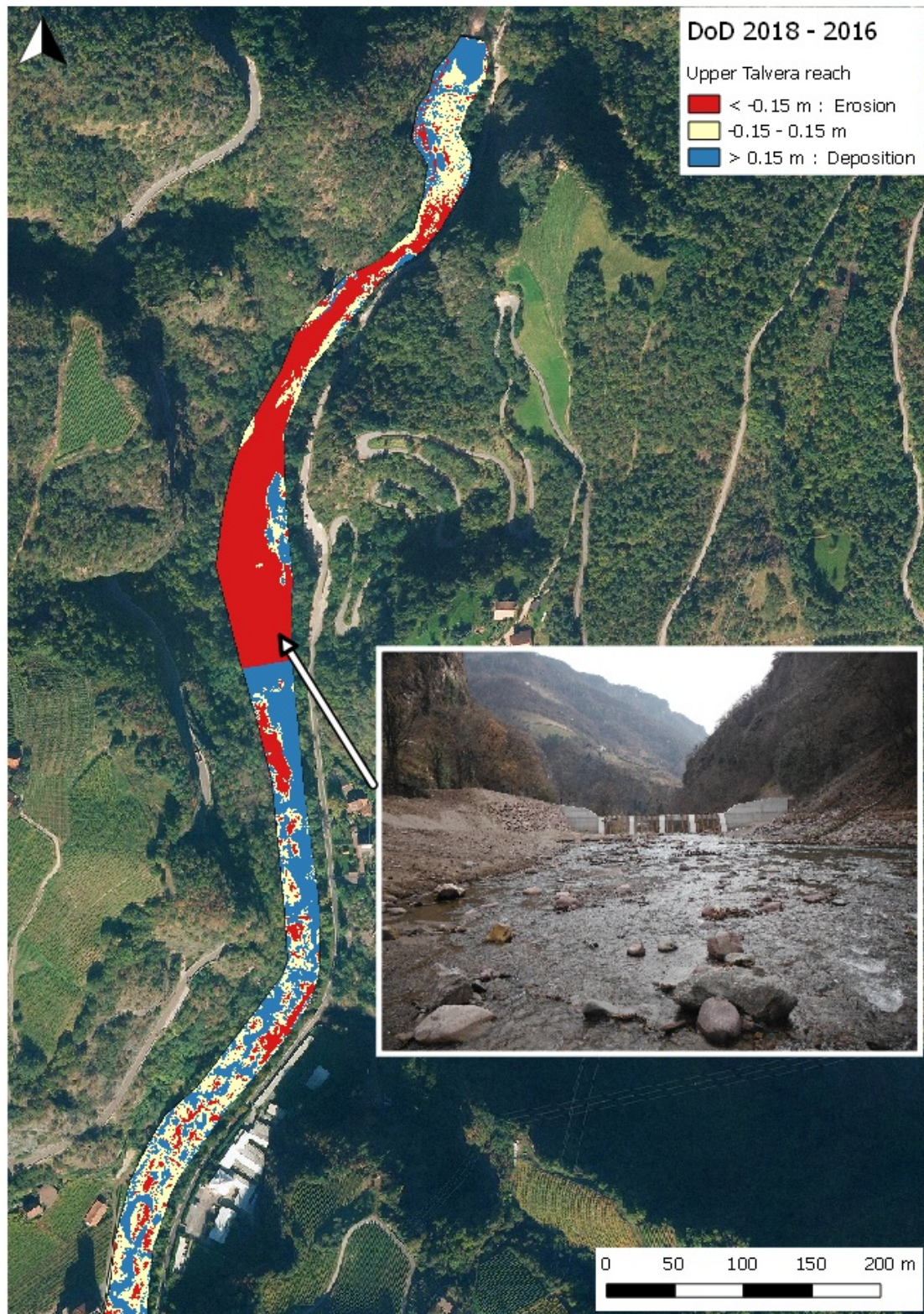
Figure 33: DoD 2018-2016 of the upper study reach of the Talvera Torrent with a picture showing erosion and deposition areas as a consequence of the check dam removal
