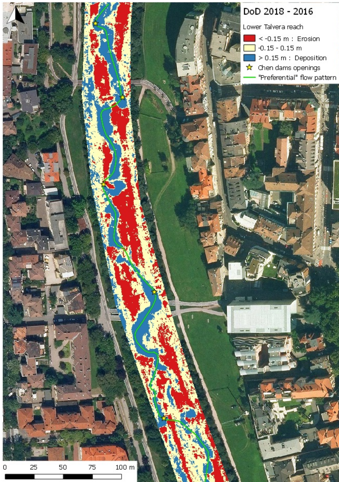
Figure 32: DoD 2018-2016 of the low study reach of the Talvera Torrent showing the depositional pattern determined by the weir openings
