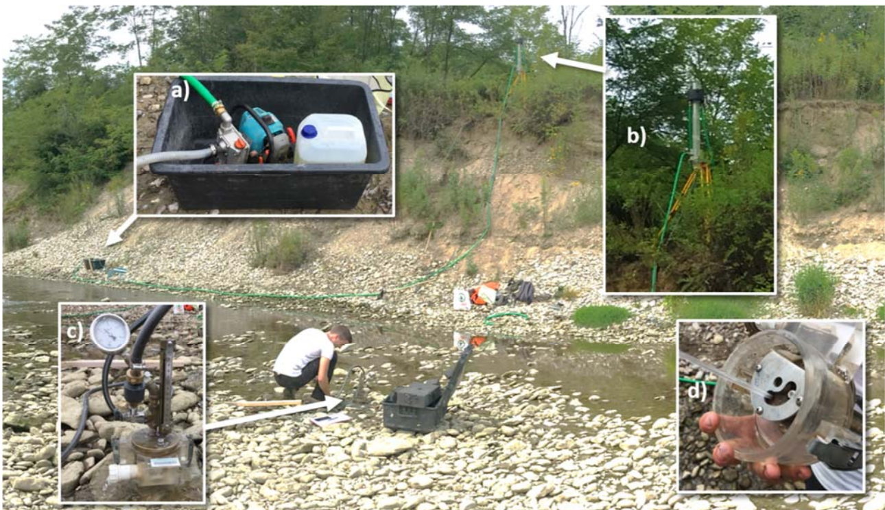
Figure 10. Instrument setup at the Mur River for deploying the Jet-test device. a) Pump continuously delivering river water to the head tank, b) head tank with continuous overflow to ensure constant water pressure at the Jet-Test instrument, c) Jet-Test device mounted on the tertiary sediment, d) Jet exiting the nozzle (submerged in water during the experiment). The Jet-test device was provided by the U.S. Department of Agriculture, National Sedimentation Laboratory, Oxford, Mississippi.
