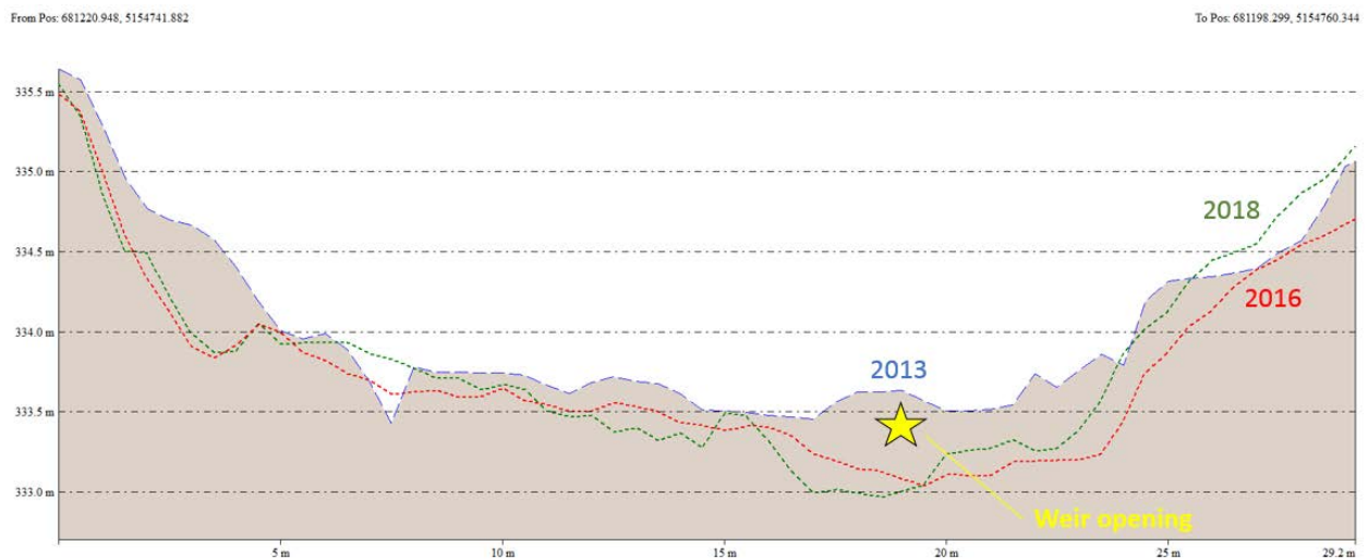
(b) Cross-section 2 showing the profile on the weir
