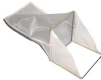
Figure 25: Example of a Surber sampler used for collecting macroinvertebrates
