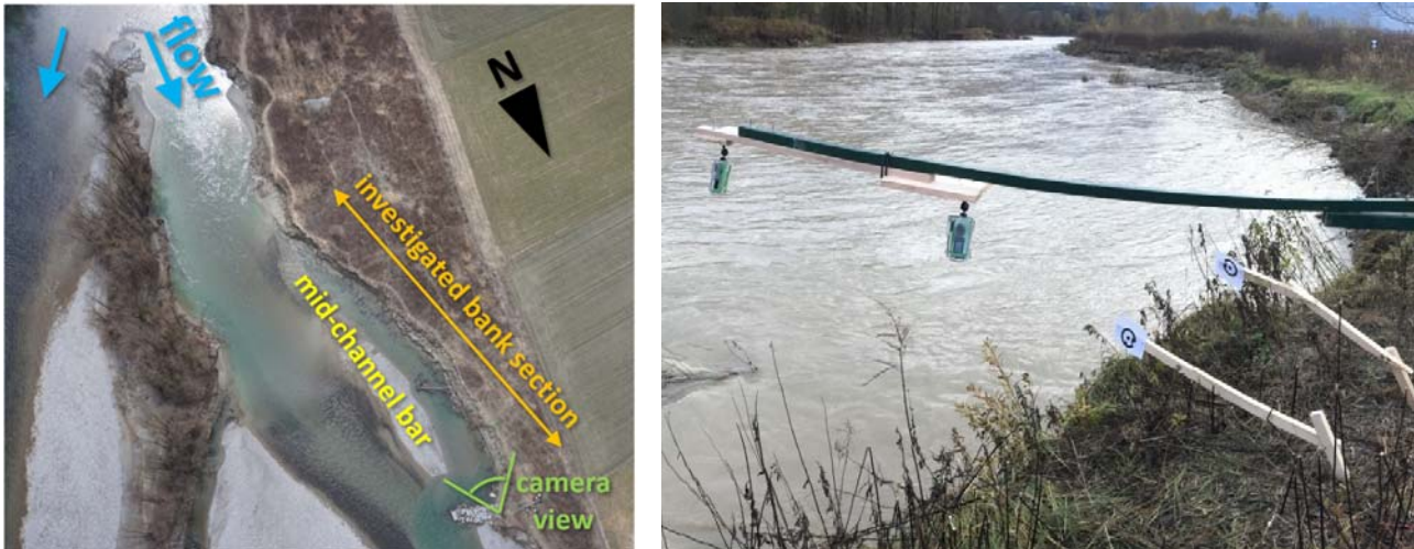
Figure 9. Left: Localisation of the investigated riverbank and mid-channel bar section including direction of the cameras' view, right: Time-lapse cameras mounted on the Drau riverbank to continuously observe the occurring bank retreat
