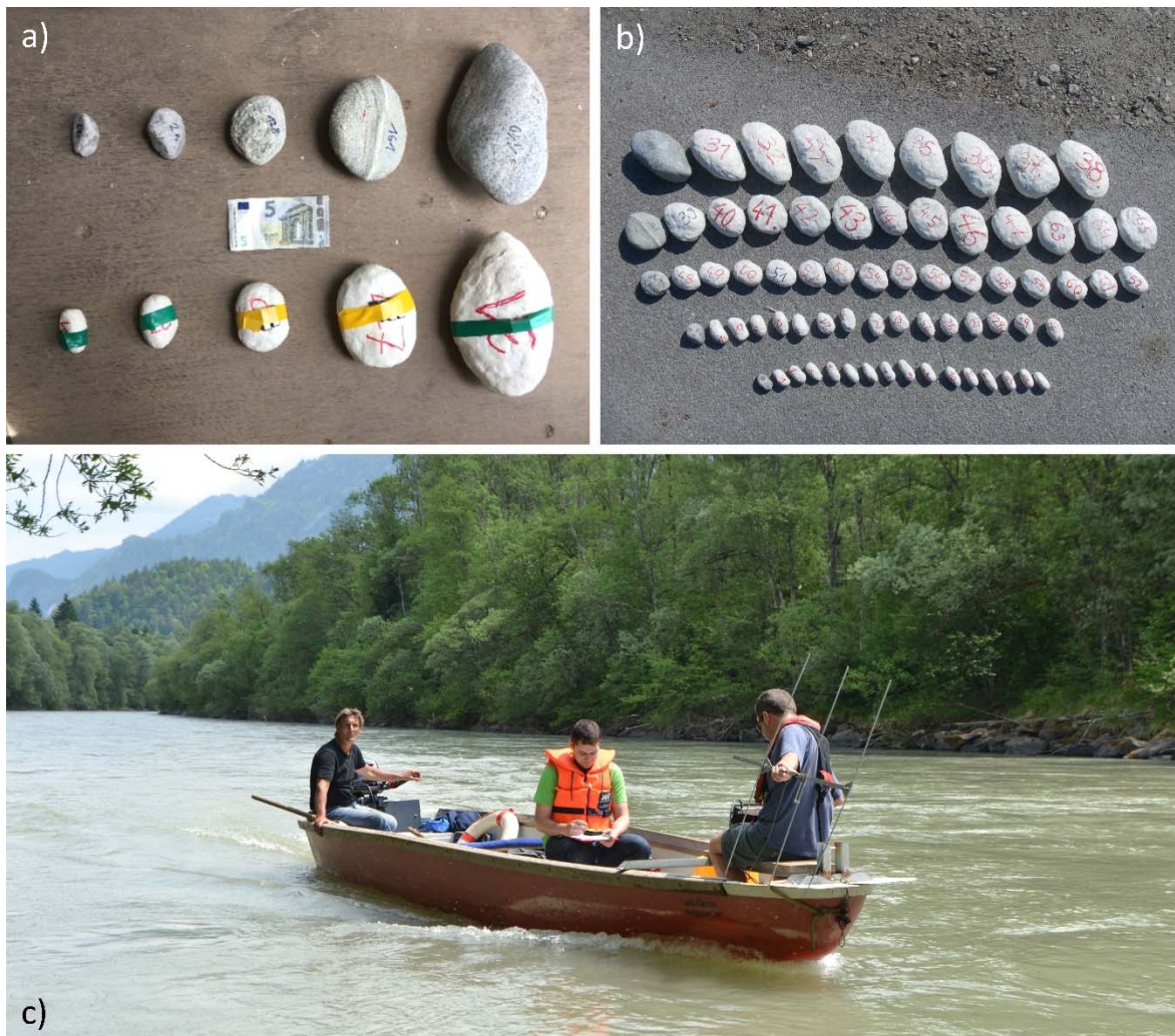
Figure 8. a) Original stones and tracer replications, b) All 65 coded radio tracer stones positioned next to the originals before insertion into the Drau River, and c) the process of searching the tracers by boat.
