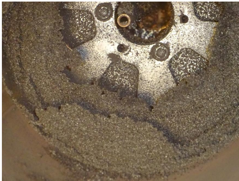
Figure 4: A picture of the reactor inside, taken from the exit of the drum. It represents the beginning of the heated reactor zone, where clearly visible the bran biochar accumulated
