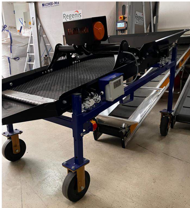
Figure 1: The 16x16 mm sieve apparatus made by FleXiever located at BEST, used to sieve sample 10
