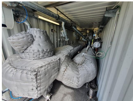
Figure 7: left: Pilot Scale pyrolysis plant from outside; right: pyrolysis plant inside container, pyrolysis reactor on left and gas burner on right side
