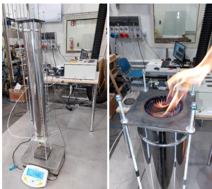
Figure 12: Lab-scale gasifier – mounted on weighing scale (L), during operation (R)
