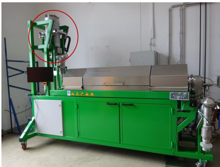
Figure 3: The used rotary kiln system, with the residue storage marked in red.
