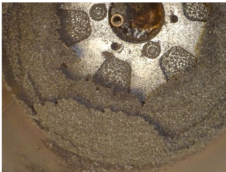
Figure 5: A picture of the reactor inside, taken from the exit of the drum. It represents the beginning of the heated reactor zone, where clearly visible the bran biochar accumulated
