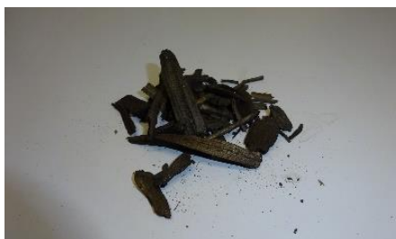
Figure 3: Biochar produced from pyrolysis of wood chips
