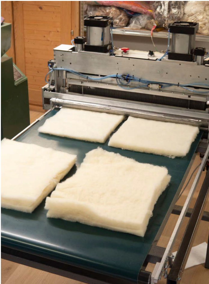
Carded wool batts entering the machine to be needle felted (left). Felt sample coming out of the machine (center). Finished sample (right). Photographs taken at Pro Verzasca(CH).
