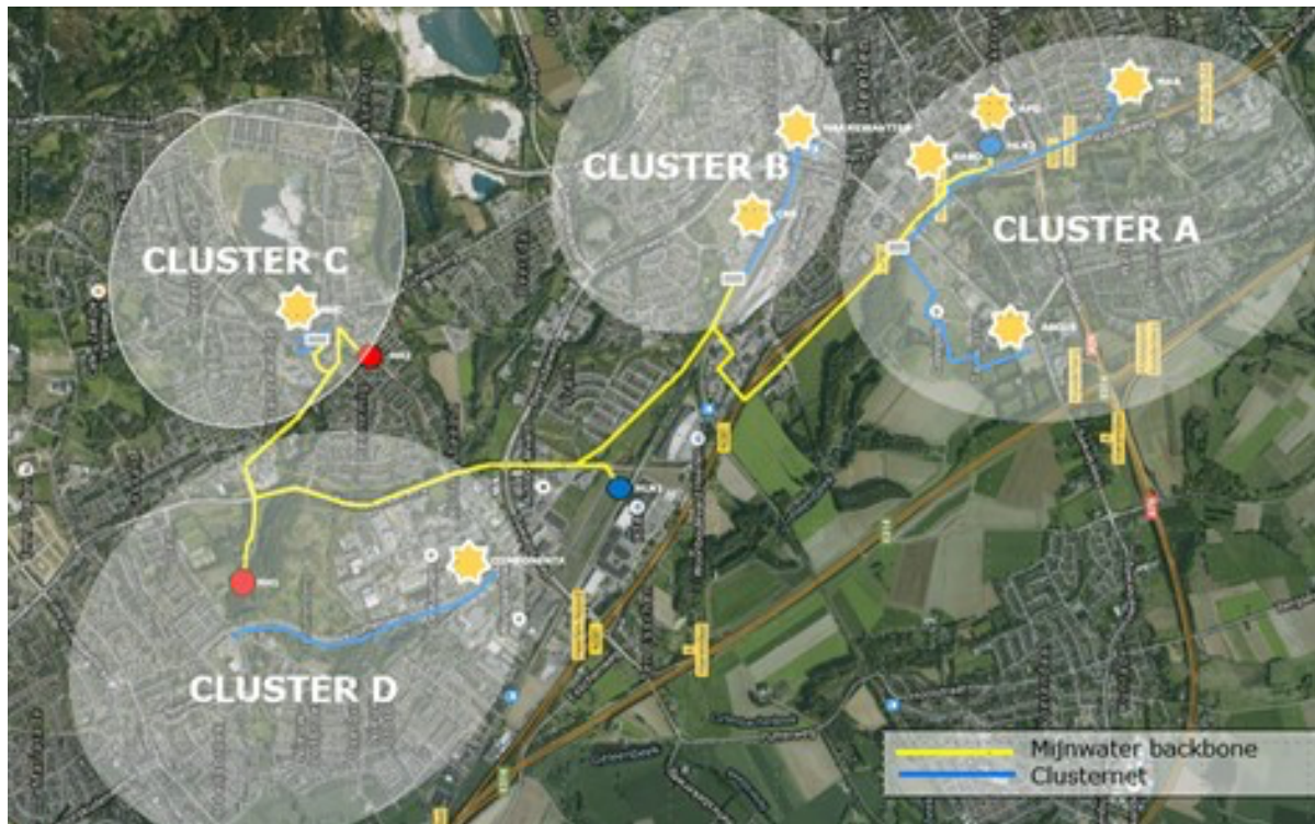
Figure 2: Schematic representation of the Mijwater 5GDHC network in Heerlen, Netherlands, depicting the cluster and backbone design. The system integrates multiple local thermal loops, each operating at ground temperature, connected via a central backbone. 9
