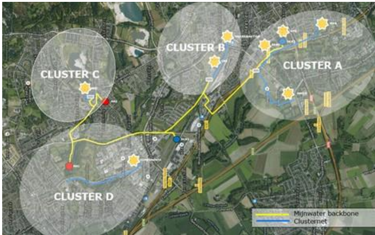
Figure 2: Schematic representation of the Mijnwater 5GDHC network in Heerlen, Netherlands, depicting the cluster and backbone design. The system integrates multiple local thermal loops, each operating at ground temperature, connected via a central backbone. 9
