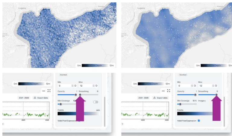
Figure 3: Spatial binning using the ‘Smoothing’ Slider in the Alplakes map viewer, for the same Sentinel-2 Secchi depth map without (left) and with 5x5 pixel binning (right).
